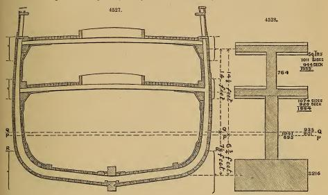
the centre line of the bottom portion, as seen in Fig. 4527. The total effective area-resisting tension is therefore 5390 sq. in., on which the above load of 11,511 tons produces a strain of  $2\frac{1}{8}$  tons a square inch.
